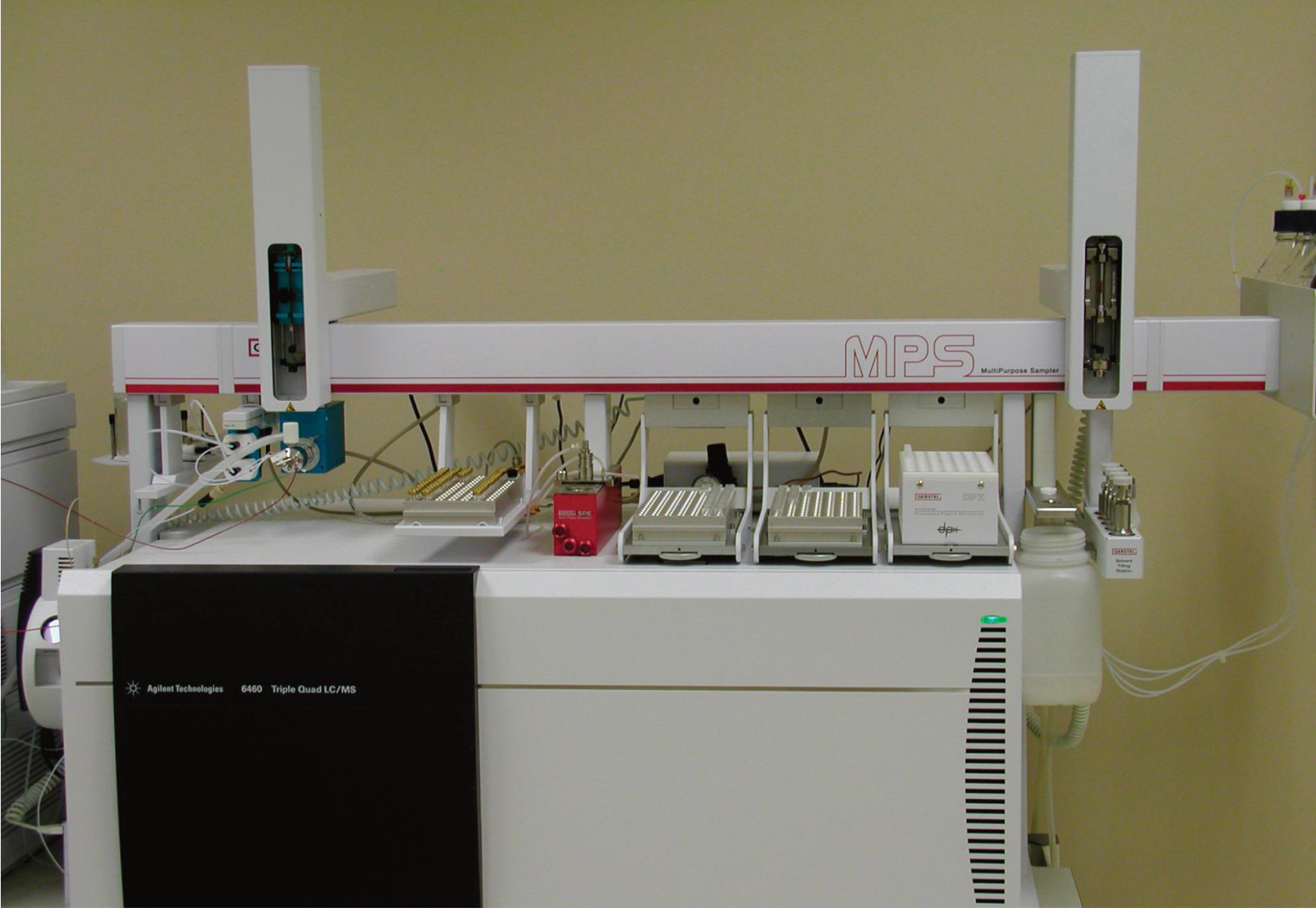
Figure 1. A picture of a GERSTEL MPS with the DPX option being used with an Agilent LC/MS/MS system. In this study, the LC/MS system was a model 6460 and the samples were extracted and eluted using 96 deep well plates.
